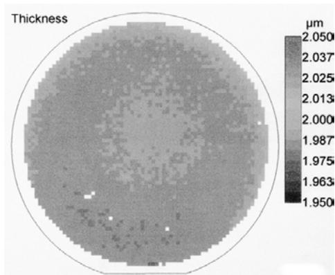
Fig. 4: Thickness uniformity of 6 inch  $\text{Al}_{0.3}\text{GaAs}$ .
