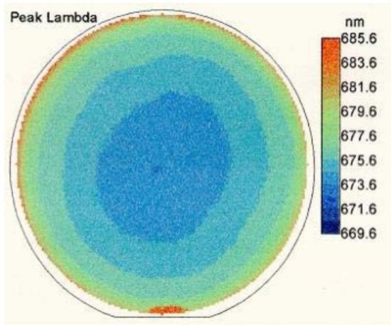
Fig. 5a: PL mapping of a 6" GaInP wafer with  $\lambda_{\text{mean}}=676\text{nm}$  and  $\sigma=1.8\text{nm}$
