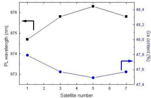
Fig. 5b: wafer to wafer distribution of PL wavelength and Ga content in a 7x6" Planetary Reactor<sup>®</sup> for GaInP
