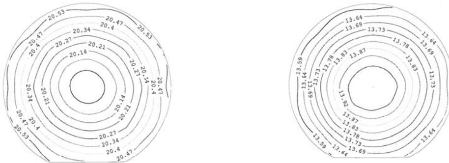
Fig. 3: On wafer doping homogeneity of 6" n-GaAs (left) and p-GaAs (right).
