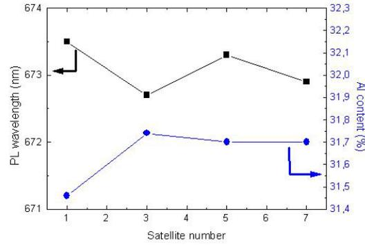
Fig. 4b: wafer to wafer distribution of PL wavelength and Al content in a 7x6" Planetary Reactor<sup>®</sup> for AlGaAs
