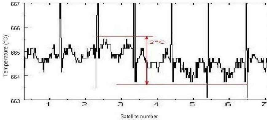
Fig.2 Wafer to wafer temperature distribution in an AIX 2600 G3 (7x6")
