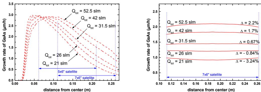
Fig. 1: Dependence of computed growth rate profiles on total flow rate in the AIX 2600 G3 7x6 inch configuration (left) on static substrates, (right) on rotated substrates.
