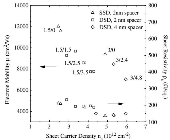
Fig. 2. Measured channel electron mobility  $\mu$  and sheet resistivity  $\rho$  as a function of the sheet carrier concentration  $n_s$  in the channel with the bottom/top silicon  $\delta$ -doping concentrations (in units of  $10^{12} \text{ cm}^{-2}$ ) and the spacer layer thickness as parameters. Data for both single-side doped (SSD, triangle) and double-side doped (DSD, square and diamond) device structures are shown.
