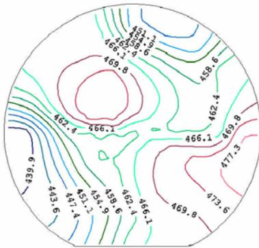
Fig.4. Sheet resistance mapping of AlGaIn/GaN HEMT on 4" sapphire substrate with 8mm edge exclusion.
