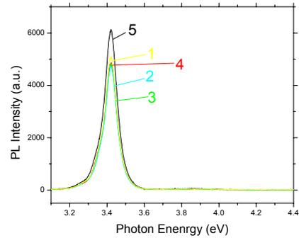
Fig. 5. Photoluminescence spectra of AlGaIn/GaN layers grown on 4" diameter sapphire wafer (#1-5 corresponds to center (1) to edge (5) with 10mm spacing between each measurement)
