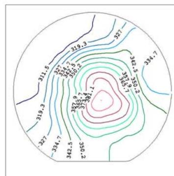
Fig. 3(a). Sheet resistance mapping of AlGaN/GaN HEMT on 3" semi-insulating silicon carbide substrate
