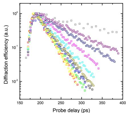
Fig. 2. Decay of light-induced grating in GaN layers with different carrier lifetimes.
