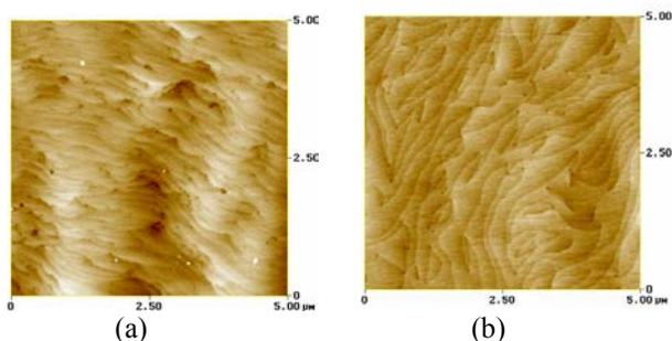
Fig. 1. Atomic force microscopic images of GaN layers grown with (a) conventional buffer layer and (b) MEMOCVD buffer layer.
