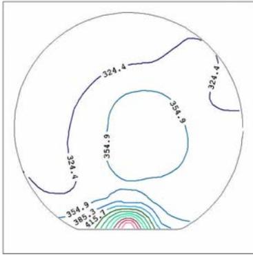
Fig. 3(b). Sheet resistance mapping of AlGaIn/GaN HEMT on 3" sapphire substrate.
