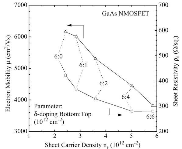
Fig. 2. Mobility (triangles) and sheet resistivity (squares) of NMOSFET structure as a function of the sheet carrier density in the channel with the concentrations of the bottom and top  $\delta$ -dopings in units of  $10^{12} \text{ cm}^{-2}$  (bottom:top) as parameter.
